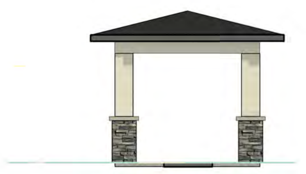
TYP. ELEVATION PET AREA PERGOLA 1/8" = 1'-0"
